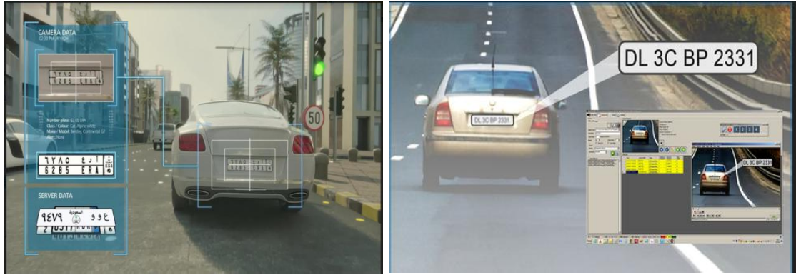
Fig.5: Number plate recognition with the help of OCR (Optical Character Recognition)
