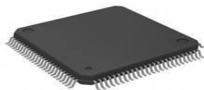
Fig.: 5 PIC Microcontroller in QFP package
